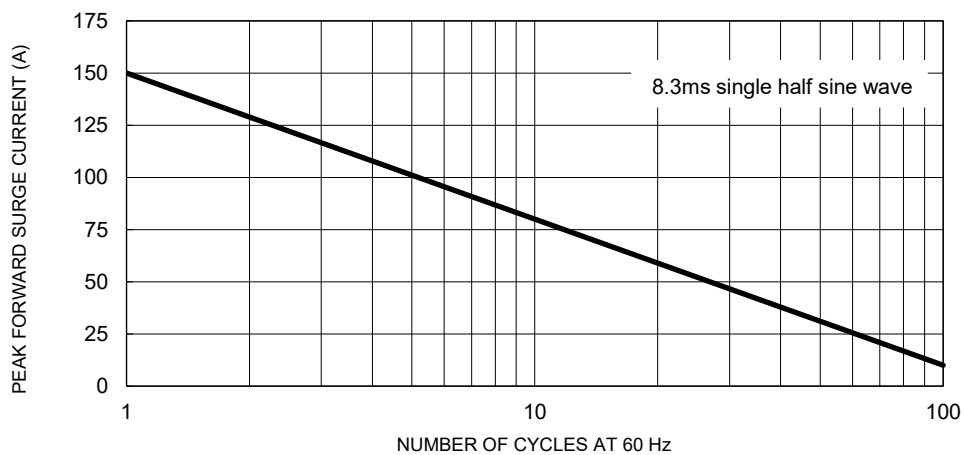
Fig.5 Maximum Non-Repetitive Forward Surge Current
